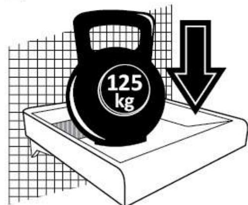
**!** This type of washbasin shall be attached to a brick or a concrete wall.
